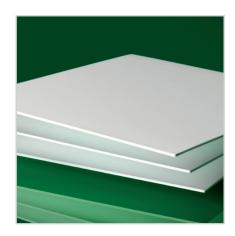
Keralpor 99 Z is required for materials reacting with  ${\rm Al_2O_3}$  and when a high evenness and purity is desired. The zirconia coating of Keralpor 99 Z prevents a reaction between  ${\rm Al_2O_3}$  and the sintered part. Additionally, due to the porous structure of the setter and coating, an adherence of the overlying ware can be avoided. This setter is preferably used to sinter Solid Oxide Cells.
