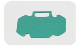
At maximum pressure, Gap Pads (SOFTTHERM® Films) should not be compressed beyond 30% of the original thickness. In case the material should be compressed more than 30%, the SOFTTHERM® material may leak out.
