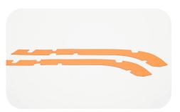
At maximum pressure, Gap Pads (SOFTTHERM® Films) should not be compressed beyond 30% of the original thickness. In case the material should be compressed more than 30%, the SOFTTHERM® material may leak out.
