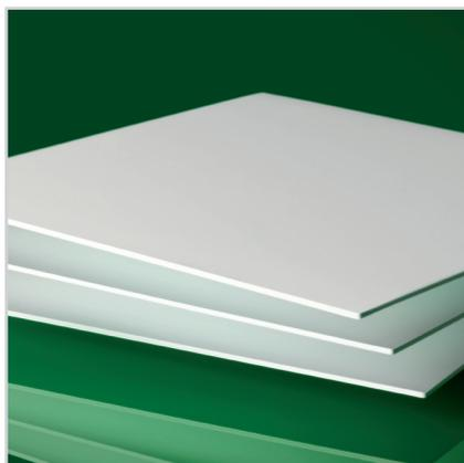
Keralpor 99 Z is required for materials reacting with  $\text{Al}_2\text{O}_3$  and when a high evenness and purity is desired. The zirconia coating of Keralpor 99 Z prevents a reaction between  $\text{Al}_2\text{O}_3$  and the sintered part. Additionally, due to the porous structure of the setter and coating, an adherence of the overlying ware can be avoided. This setter is preferably used to sinter Solid Oxide Cells.
