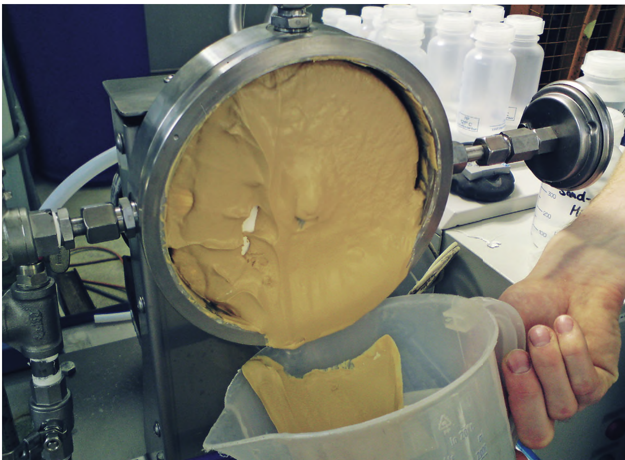
Figure 3. Example of the high viscosity that can be obtained with DCFF ©ANDRITZ KMPT GmbH. [3]
