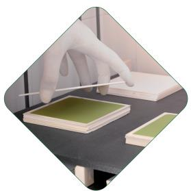
Keralpor 99 Z is required for materials reacting with  $Al_2O_3$  and when a high evenness and purity is desired. The zirconia coating of Keralpor 99 Z prevents a reaction between  $Al_2O_3$  and the part to be sintered. Additionally, due to the porous structure of the setter an adherence of the overlying ware can be avoided.
