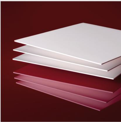
Due to the low heat capacity, the demand of energy for the kiln is lower, compared to conventional setter and kiln furniture. The demand of time and energy for heating up and cooling down the kiln furniture is significantly reduced by using Kerafol setter plates.
