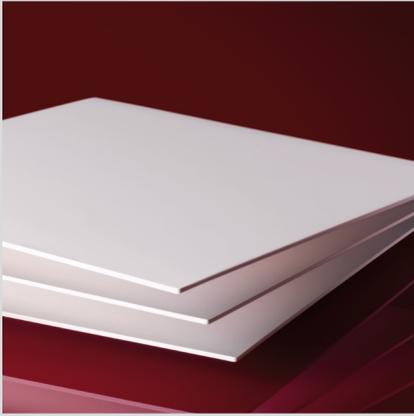
The Keralpor S is a setter, which can be used for sintering various of metal injection moulding (MIM) - products and materials. The advantage of this porous zirconia toughened alumina is its good thermal shock resistance and high mechanical strength. Through the 38% porous structure, adhesion of the sintered part will be prevented.
